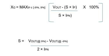
$V{\rm OUT}({\scriptstyle (@ \ IPN)} \text{ and } V{\rm OUT}({\scriptstyle (@ \ IPN)} \text{ stand for the voltage output at } IPN \text{ and } \text{-IPN respectively.}$
