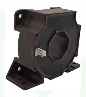
The OPCO 500 is a closed-loop current sensor (also known as a compensated current transducer), designed for the precise measurement of AC and DC currents up to 500A. This sensor uses Hall Effect technology in a closed-loop configuration, providing high accuracy and excellent linearity in the measurement of both alternating and direct currents.
