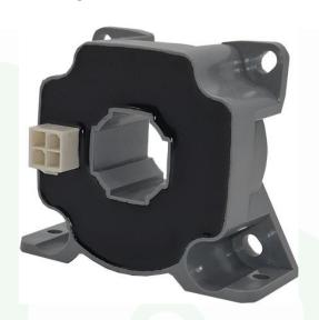
The OPCO 300 is a closed-loop current sensor (also known as a compensated current transducer), designed for the precise measurement of AC and DC currents up to 500A. This sensor uses Hall Effect technology in a closed-loop configuration, providing high accuracy and excellent linearity in the measurement of both alternating and direct currents.
