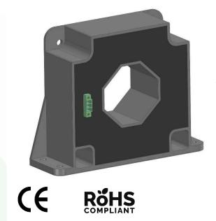
The OPCO 2000 is a closed-loop current sensor (also known as a compensated current transducer), designed for the precise measurement of AC and DC currents up to 2000A. This sensor uses Hall Effect technology in a closed-loop configuration, providing high accuracy and excellent linearity in the measurement of both alternating and direct currents.
