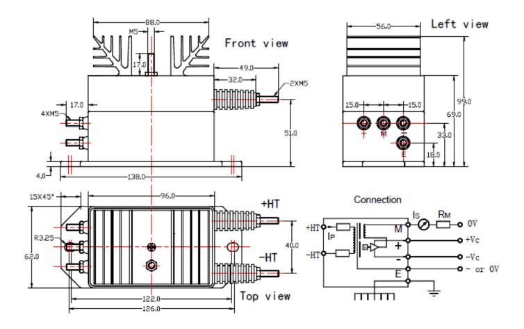
All dimensions are in : mm General Tolerance : ± 1mm
