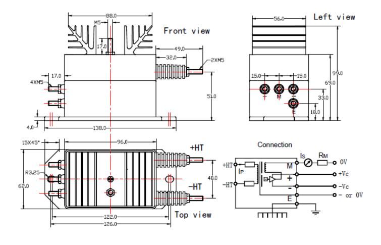
All dimensions are in : mm General Tolerance : ± 1mm Primary connection : M5 threaded studs Tightening torque : 2.2 N.m Secondary connection : M5 threaded studs Tightening torque : 2.2 N.m
